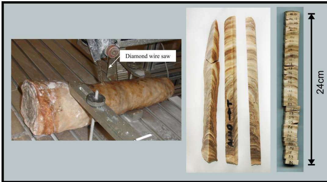
Figure 4.1: Sample Alho 6 from the Pau D'Alho cave; left , diamond wire-saw used to separate the stalagmite in two halves; middle , three slabs obtained; right , 34 discrete specimens obtained using a common rock saw.
