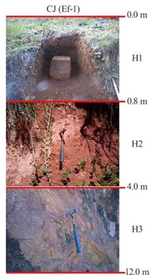
Figure 3.12 – Soil profile from geotechnical investigation (Mendes et al., 2015).
