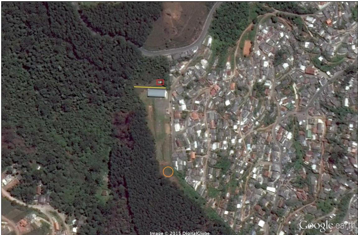
Figure 3.4 – A Google Earth satellite image of the site of investigation. The geophone array is represented by the yellow line, the caged monitoring station by the red box, and the orange circle represents the location where the passive MASW survey was performed.
