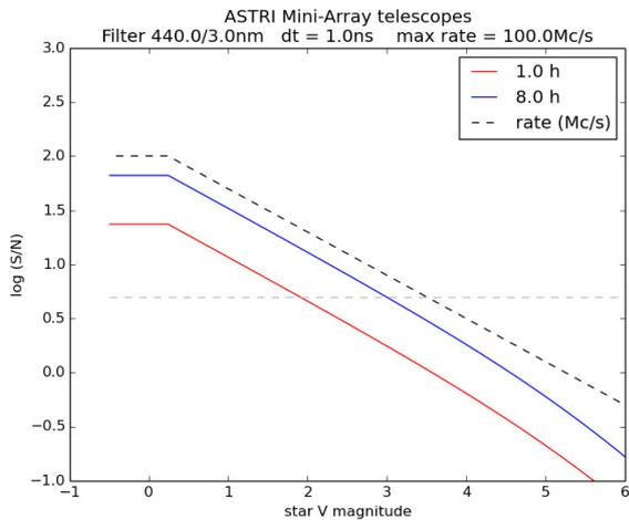
**Figure 45:** S/N ratio for a SII measurement with two ASTRI Mini-Array telescopes as a function of stellar magnitude. The source photon flux is limited in order to give a maximum rate of 100 Mcounts/s. The simulation is done using a narrow-band filter centered at 440 nm and with a FWHM of 3 nm (plus a polarizer). The bin time is 1 ns and the observing time is 1 hr (red line) and 8 hrs (blue line). The gray dashed line corresponds to  $S/N=5$ .
