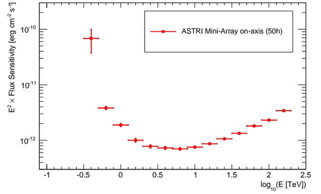
**Figure 4:** On-axis differential sensitivity (multiplied by energy squared) of the ASTRI Mini-Array for 50 hours of observations as a function of the energy between  $\approx 0.3$  TeV and  $\approx 200$  TeV.
