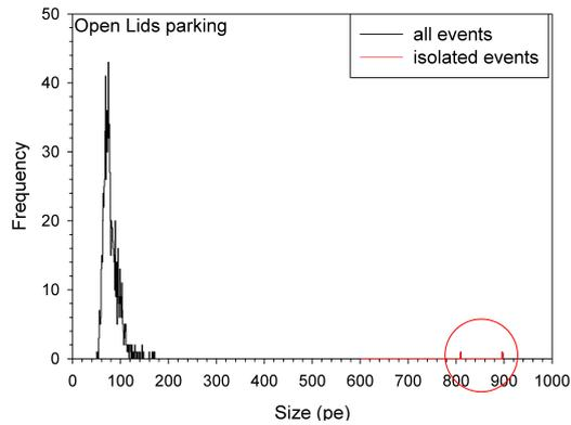
**Figure 41:** Size distribution of all the events detected in the six minutes run. The size is calculated, event by event, summing the image-pixels greater than 12 pe. Isolated events are shown in red.
