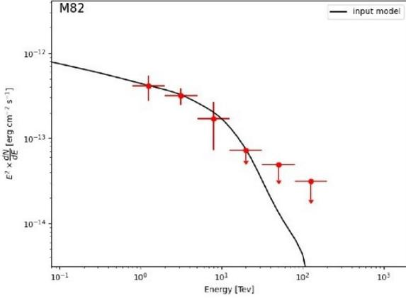
**Figure 24:** Simulated  $\gamma$ -ray spectrum of M 82. Red points represent the signal that can be observed by ASTRI Mini-Array after 100 hours of observation, and assuming the spectrum predicted by the starburst model (black line, Peretti et al. 2019). The spectral points and their error bars are obtained from the distribution of 100 simulations.
