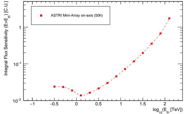
**Figure 5:** On-axis integral sensitivity of the ASTRI Mini-Array for sources with a Crab Nebula-like spectrum for 50 hours of observations as a function of the energy threshold in the range between  $\approx 0.3$  TeV and  $\approx 150$  TeV.
