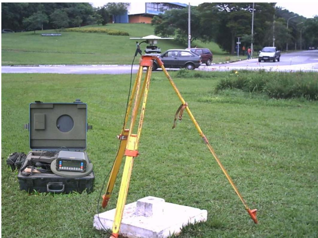
Figura 3.5 – Receptor, ASHTECH Z12 e antena ASHTECH ASH700718A
